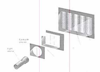
The light bends as it passes through the slits (diffraction) and shows light bands (constructive interference) and dark bands (destructive interference).
